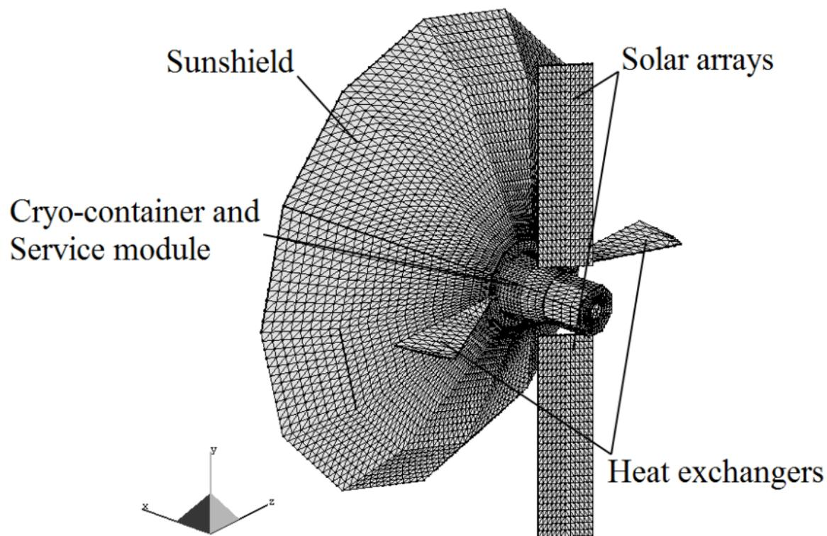
Figure 7: Geometrical model of Millimetron space observatory.
